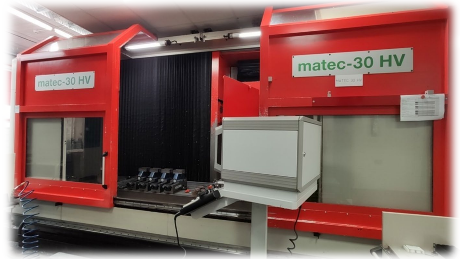
CNC-bed milling machine MATEC, 4-axes X 3000mm, Y 800, Z 800
