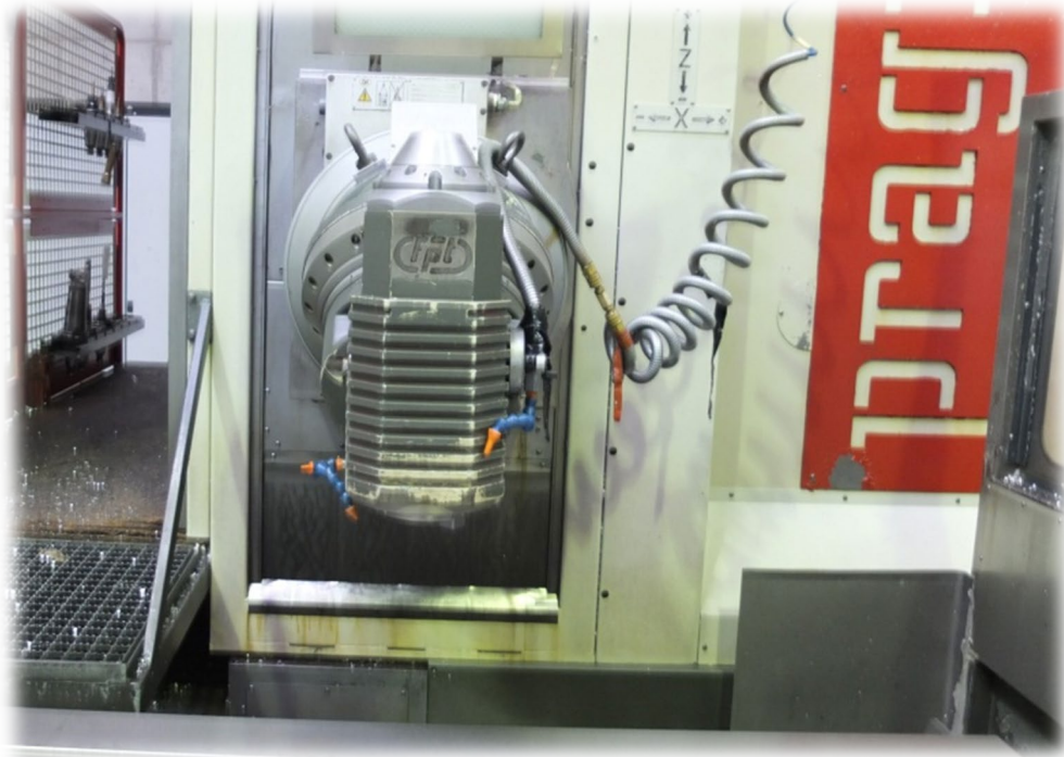
CNC-traveling column MC FPT X 6000mm, Y 1200, Z 2300
