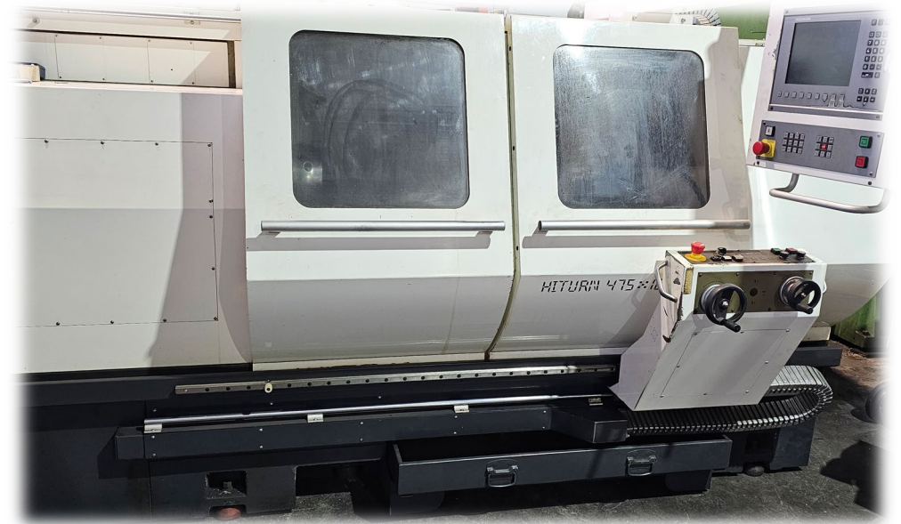
Cycle lathe WEMAS X 2000mm, Z 400
