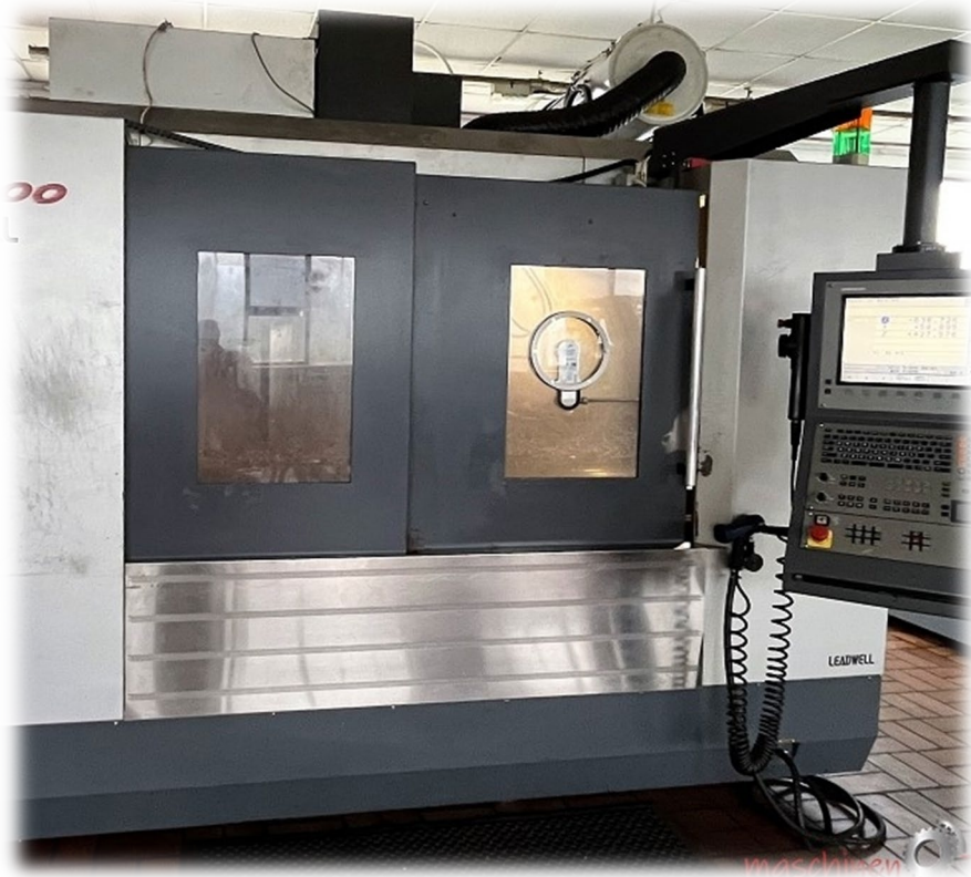
CNC-MC vertically LEADWELL X 1300mm, Y 635, Z 610
