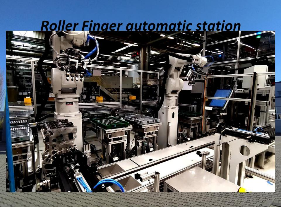
Cylinder Head screw loading station
