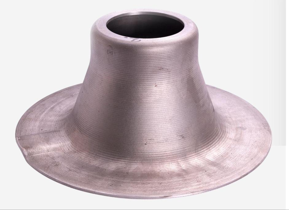
Metal spinning is a precision forming process that transforms flat metal into strong, seamless, symmetrical and durable components. At Bratstvo by using controlled rotation and forming tools, we achieve flawless shapes, minimal waste and superior strength. Unlike other metal-forming methods, spinning creates strong parts without the need of welding or joints, reducing the risk of structural weaknesses.
