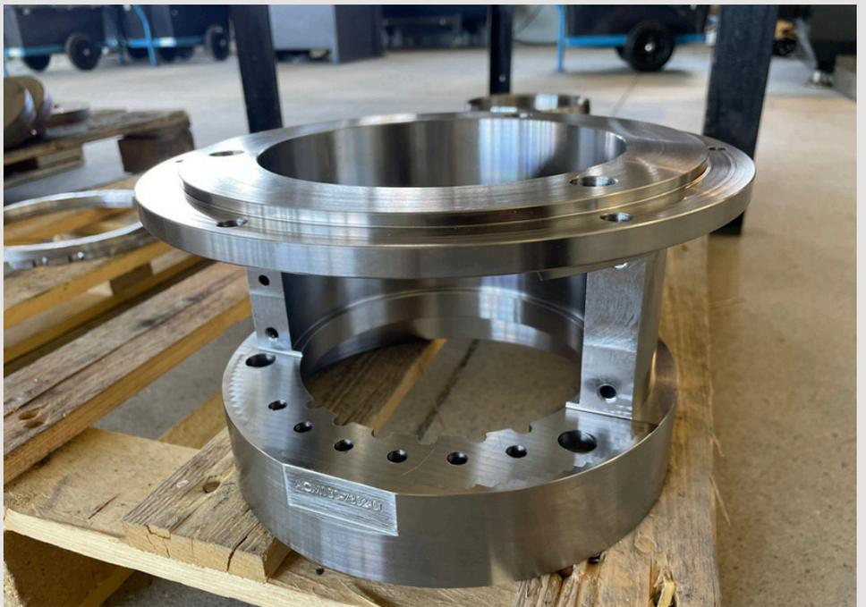
THE LAST PART HAS BEEN MILLED AFTER TURNING OPERATIONS. OUR TURNING MACHINES INCLUDE Y AXES FOR MILLING OPERATIONS.
