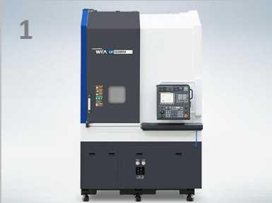
HYUNDAI LV800 VERTICAL TURNING CENTRE Z: 700 Ø 800
