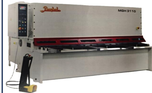
Baykal MGH 3100 × 10 Guillotine Shear Hydraulic swing beam design
