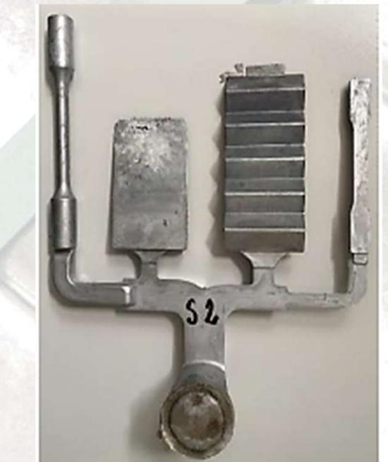
Silafont-36 Test on prototype tool
