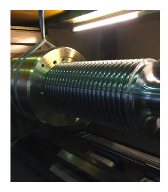
We specialise in the production of spare parts and the maintenance of components that can be installed in original equipment quality. We repair damaged or obsolete components or restore them if necessary. We are able to process them with lengths of up to 20 metres and unit weights of up to 30 tonnes.
